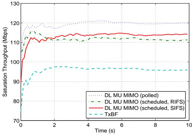
Fig. 10. Saturation throughput  $S$  (without MAC protection).
