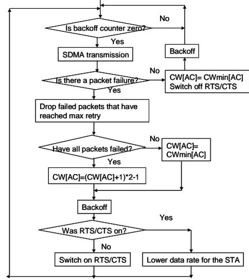
Fig. 4. Flow chart of the AP backoff procedure.
