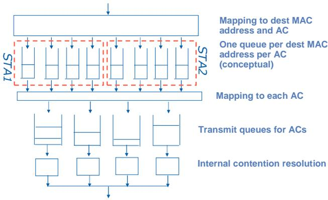
Fig. 6. Illustration of Weighted Queuing at the AP.
