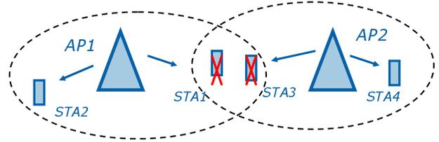
Fig. 5. Illustration of a hidden node scenario.
