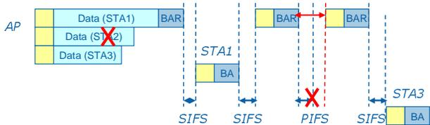
Fig. 3. Error recovery for polled response mechanism.
