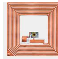
Figure 1: A passive NFC tag with 2K bytes of memory.
