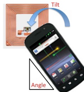
Figure 2: A smart phone reading a tag while being tilted to define an analog parameter that can control a remote device.
