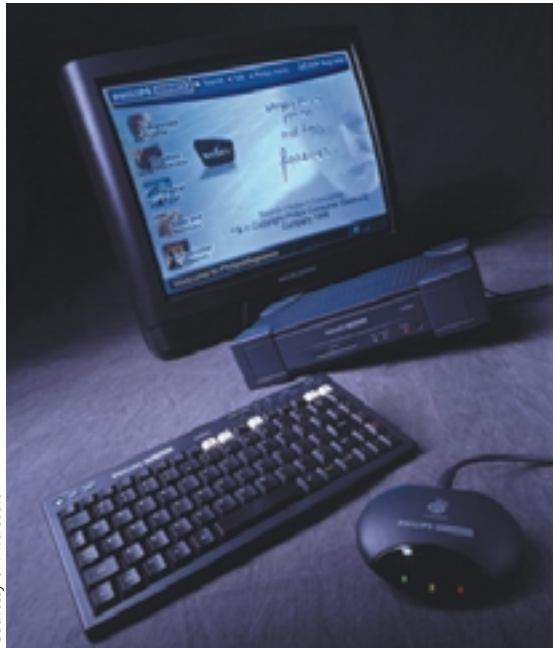
4 Components of WebTV (from top to bottom): a TV set, a set-top box, a keyboard, and an input-control device.
