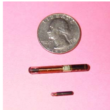
Figure 2. A Trovan RFID tag [base] weighs from 0.1 (grain of rice size) to 7 grams (credit-card size), and contains a 39-bit unique identifier.
