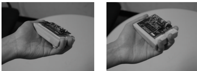
Fig. 2. Tilting a small device. Pictured is a user tilting up and then returning to center.
