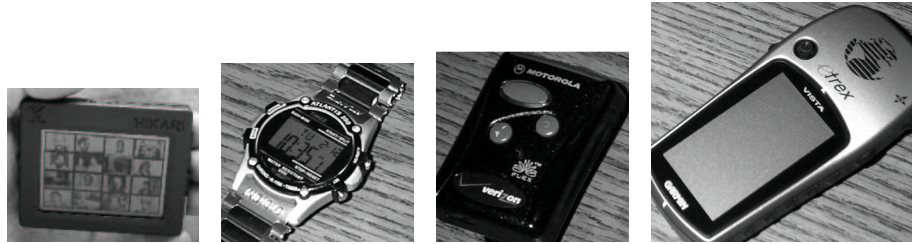
Fig. 1. Small devices with few or no buttons and varying amounts of screen space. User input on such devices can be very awkward. Pictured is the Hikari, a Timex Atlantis 100™ watch (approx. 41mm in diameter), a Motorola™ BR850 pager (approx. 60 × 40 × 15 mm), and a Garmin eTrex Vista™ GPS receiver (112 × 51 × 30 mm).
