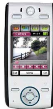
Fig. 5. The Motorola e680i multimedia cell-phone platform, supporting both A2DP- and PAN- based wireless streaming over Bluetooth.
