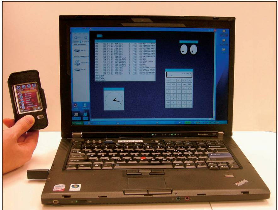
Figure 2. A Linux/XScale-based cell phone renders its desktop wirelessly to a nearby PC with a full-size display and keyboard, thus enabling effective user interaction.
