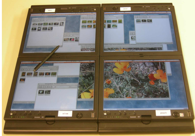
Fig. 1. Four individual tablet computers, linked only by a wireless network, forming a multi-display composition resulting in a single logical display.
