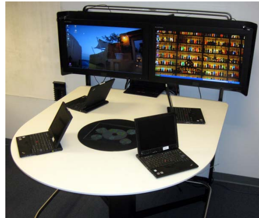
Figure 1: A collaborative workspace table prototype, showing four laptops, two embedded displays, and a central embedded control surface.
